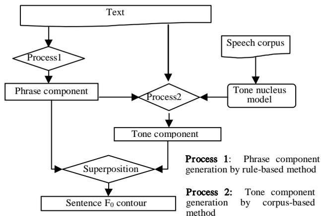
Figure 1: Two-step scheme of  $F_0$  contour generation.
