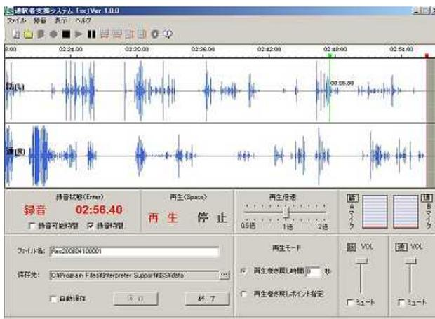
Figure 2: User Interface for the system. The speech waveforms of an original speaker and an interpreter are respectively shown in the upper and lower windows. The part being played is indicated by a green cursor in the upper window. The replay speed can be changed between the rates of 0.6 times and 2.0 times at intervals of 0.2 times. The users can speed up or slow down the replay at any given point in time.
